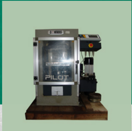
3,000 KN Concrete compressive Machine in fixed and mobile laboratories
