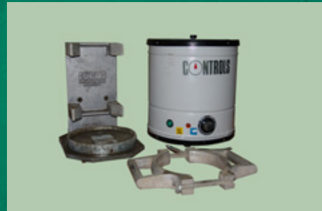
Concrete cores sulphur capping equipment
