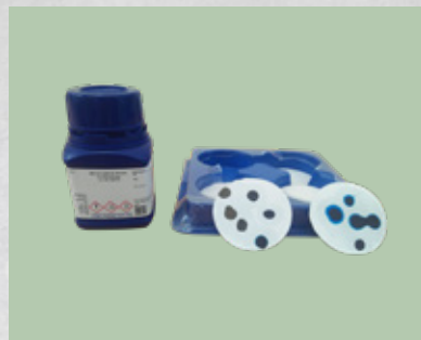
Methylene Blue Value (MBV) test apparatus for clay content determination
