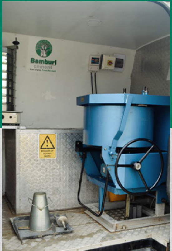
Concrete mixer and slump equipment in mobile concrete laboratory
